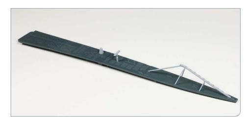
The capstan has now been mounted on the foredeck, and the two sections of the upper deck are joined together.
