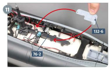
Take the guide rail 132-6 and place it onto the guide 76-2, so that the holes of the two parts are aligned.
