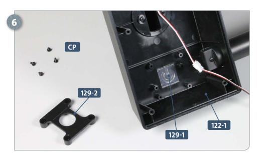
Insert the power button 129-1 into the slot on the underside of the forward stand section 122-1. Have ready the mounting bracket 129-2 and four CP screws.
