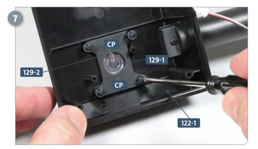
Fit the mounting bracket 129-2 into the body of the stand 122-1, so that it holds the power button 129-1 in place. Secure the mounting bracket to the stand section with the four CP screws, as pictured left.
