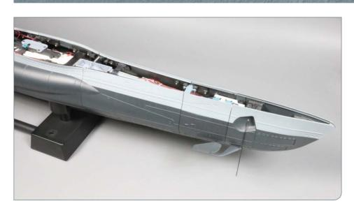
Both forward dive planes have now been attached, along with their protective brackets. The forward torpedo loading bay and box have also now been installed on the deckhead.
